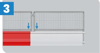
The leg of the fence panel doubles-up as a support strut to hold the corner angles/barriers in place.
