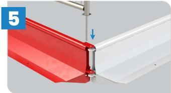
Corner barriers can be attached to the standard barriers. Simply line up the ends and insert the connecting or fence panel lea.
