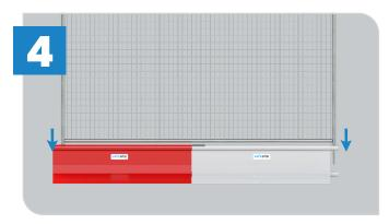
With the connecting pin in place, you can then slot the fence panel legs into place so that it straddles 2 consecutive barriers.
