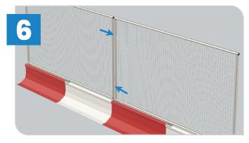
2 Standard Couplers should be used to secure the Fence panels together.
