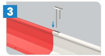
Once the barriers are in place, the connecting pin slots down through the top of the barrier to hold in place.
