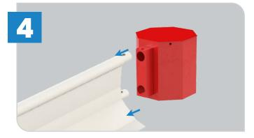
To finish the barriers in a line butt the end stop into the end of the barrier.
